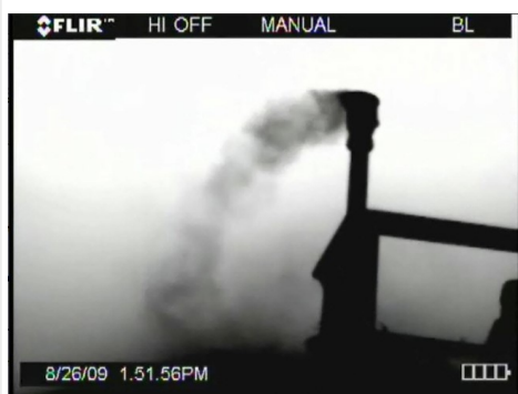
Infrared image of emissions from a natural gas storage tank Source: Texas Commission on Environmental Quality
